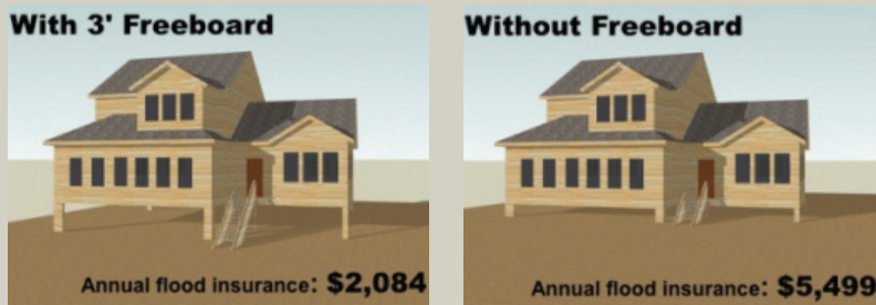
Figure 2-7. Adding a small amount of height has very little effect on the look of a home but can pay dividends in flood protection. Source: Louisiana Storm Smart Coasts.
