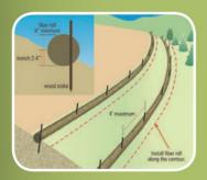
Illustration of filter log installation.
