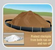
Application of silt fencing to control muddy runoff from soil stockpile. Leaving a site with quality soil encourages healthy root growth and reduces time and resources needed to care for turf and landscape plantings.
